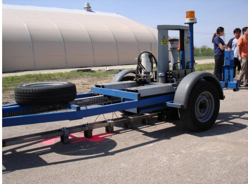
Figure 2.1. Dynatest Falling Weight Deflectometer device.
