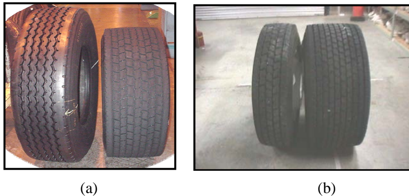
Figure 1.1. (a) Comparison between the First and New Generations of Wide-base Tires, and (b) Comparison between a One Tire in Dual-tire Assembly and a New-generation Wide-base Tire.
