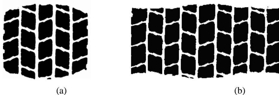
Figure 2.1. Tire Imprint Area for (a) One Tire of a Dual-tire Assembly and (b) New Generation of Wide-base Tire (after Al-Qadi et al. 2005).
