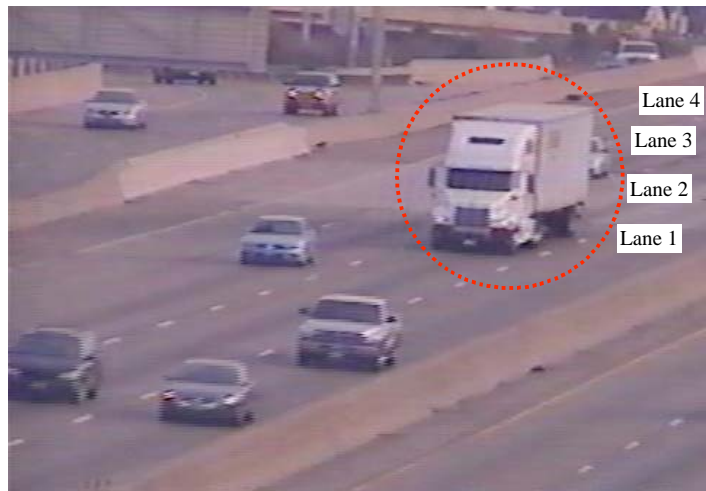
Figure 5.1, An example of drop-out without return (DOWoR) from a long vehicle in lane 2 during the 29 min of ground truth (17:21 to 17:50) on 3/09/2009.
