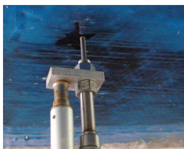
Figure 3-8 Installation of LVDT
