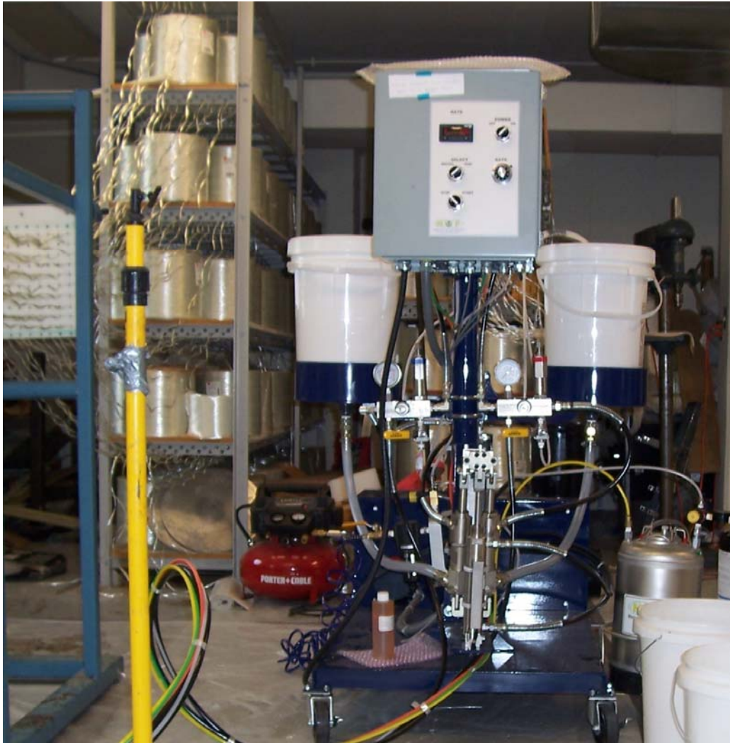
Figure 1. Metering unit setup for pultrusion process
