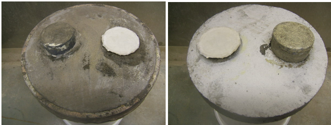
(a) Before Spraying Curing Compound
