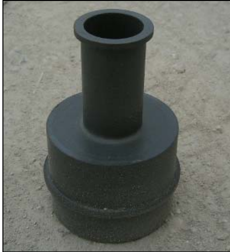
Figure 3-8. Chilled Mirror Chamber.
