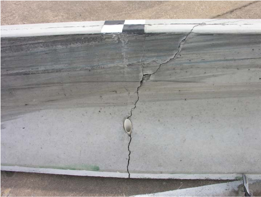
Figure 27. Barrier No. 5 Damage, Test NYTCB-4
