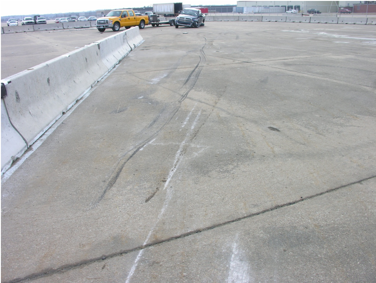
Figure 24. Vehicle Final Position and Trajectory Marks, Test NYTCB-4
