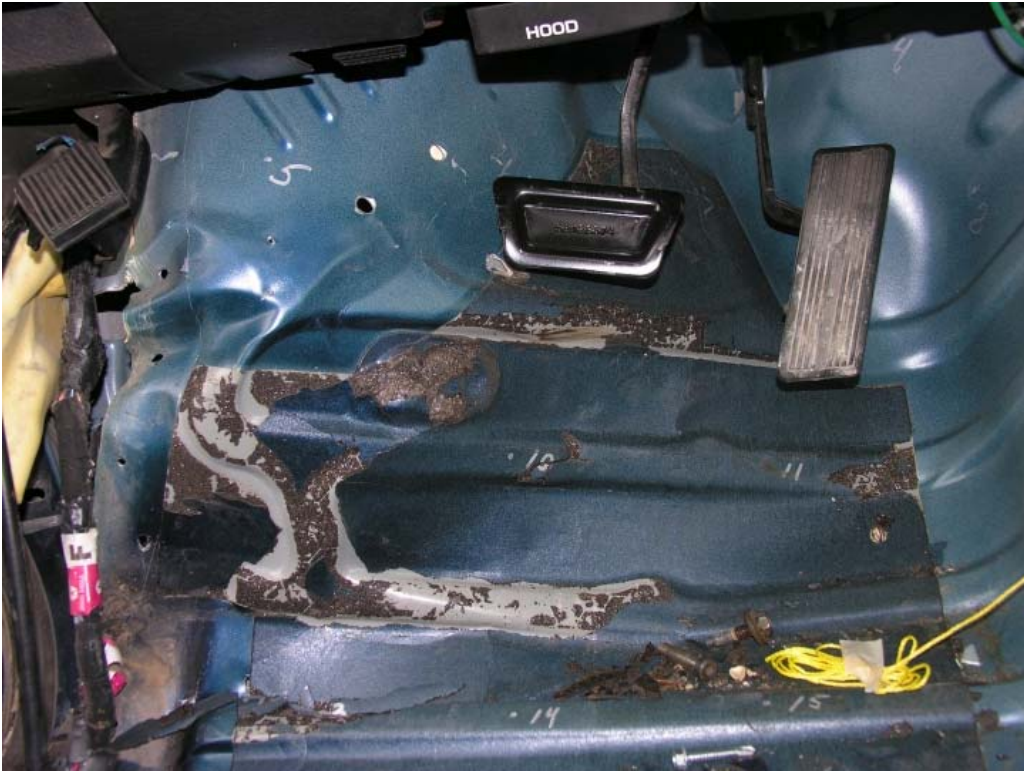
Figure 37. Occupant Compartment Deformation, Test NYTCB-4
