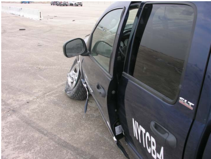
Figure 35. Vehicle Damage, Test NYTCB-4
