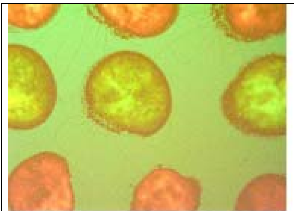
Figure 54: Optical microscope image of an QD array of different sizes or colors
