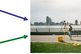
**After CORS:** Accurate differential GPS positioning with one-person field crew.
