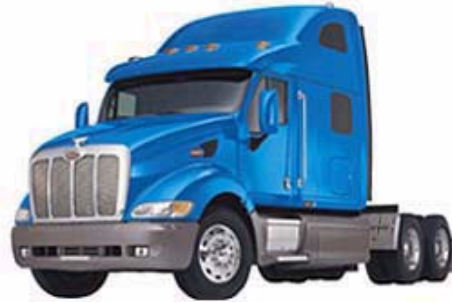
Aerodynamic conventional tractor with integrated cab-roof fairing. (Peterbilt 387)
