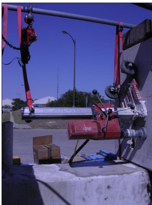
Figure 4-33: Second Series Specimens - Extraction of Cores
