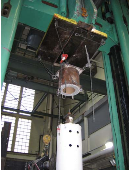
Figure 3-3. Loading ring above specimen.
