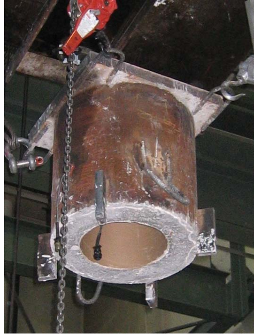
Figure 3-4. Close up of loading ring
