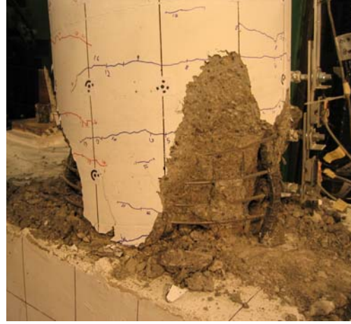
Figure 4-9. LB7-PT: Bar V18, Cycle 37 (-9.55%).
