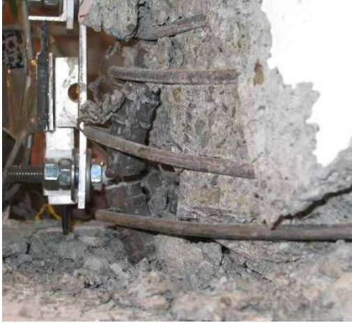
Figure 4-8. LB7-PT: Bar V00 fracture, Cycle 35 (2.11%).
