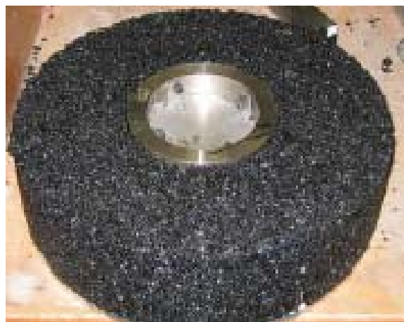
Figure 5.1 ACCD ring (at the center) with HMA compacted outside.
