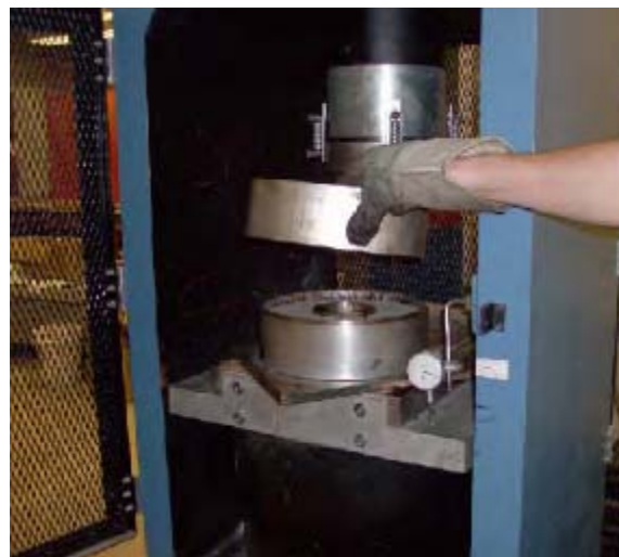
Figure 5.3 ACCD concentric ring short mold (variation 2) after compaction.
