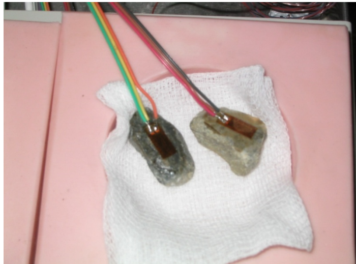
Figure 3.1 Strain gages instrumented on the polished aggregate surfaces.
