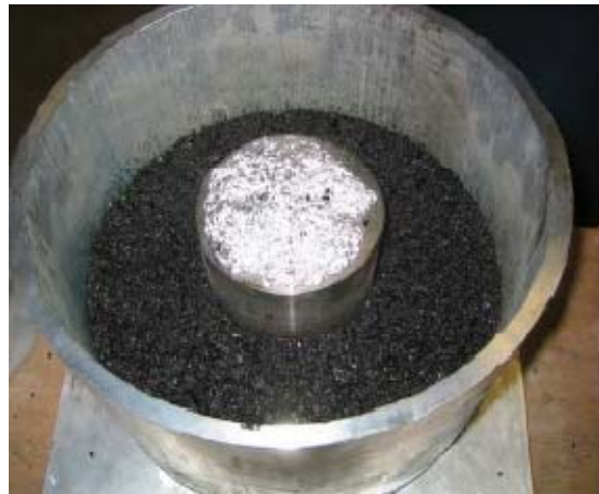
Figure 5.2 Concentric ring ACCD long mold (variation 1) after compaction.
