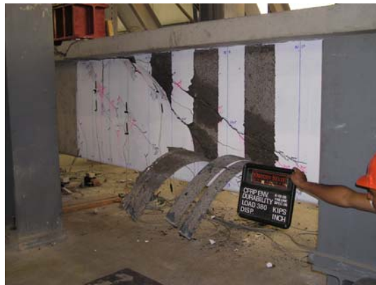
Figure 5.19: Failure photograph of Specimen IT12FTCK
