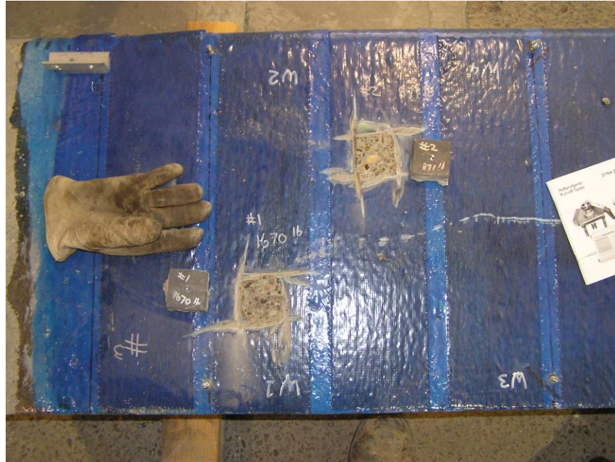
Figure B-4.4: Cohesive failure of concrete surface bonded to CFRP caused by direct-tension pull-off tests
