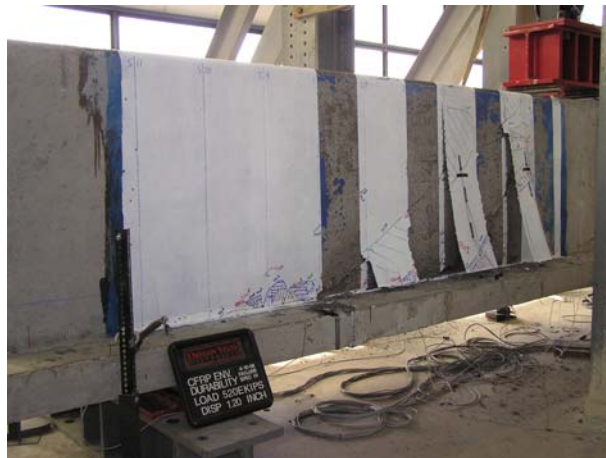
Figure 5.14: Failure photograph of Specimen IT12M
