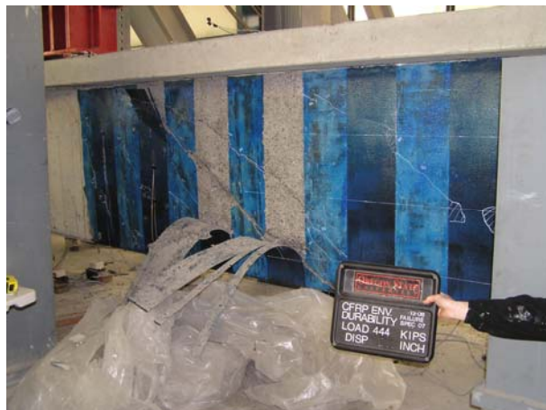
Figure 5.17: Failure photograph of Specimen T18Control
