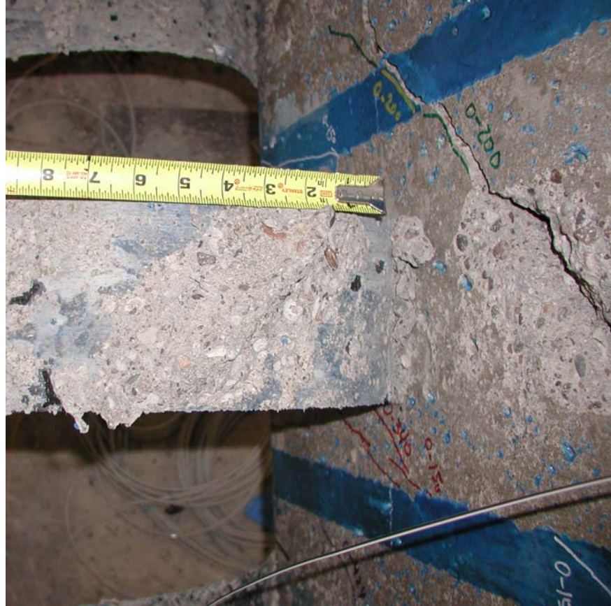
Figure B-5.7: Photograph of a debonded CFRP strip that formerly crossed a diagonal crack (post-failure of Specimen FC)
