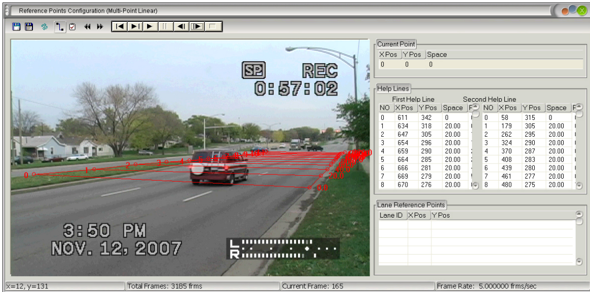
Figure 8: Extracting Vehicular Trajectory Data over Yellow Interval by Using VEVID
