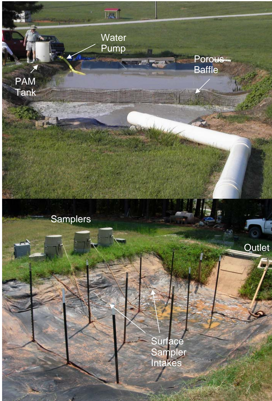
Figure 1-1. Layout of the experiment showing the mixing basin (top) and the open stilling basin with no baffles (bottom).
