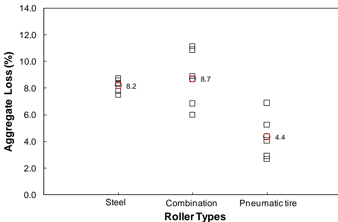
Figure 4-3 Aggregate loss of a straight seal obtained from FOT samples
