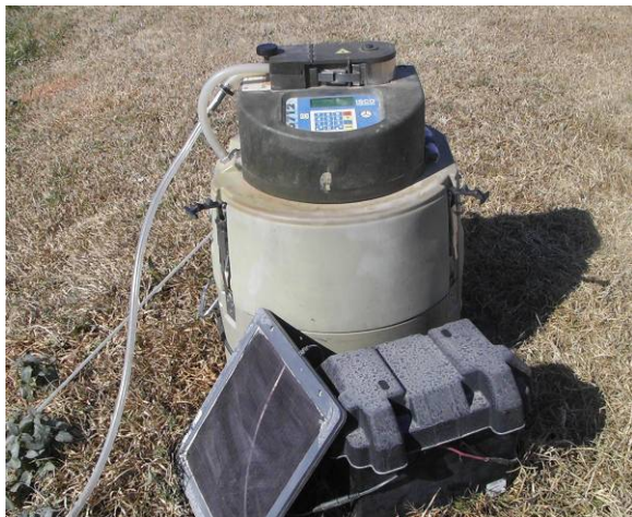
Figure 10. ISCO water sampler.
