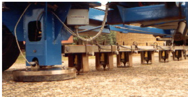
Figure 2. FWD Load Plate and Sensors
