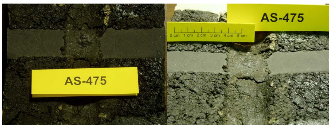
Figure 13 Photograph of APA Test rutting results of AS 475.
