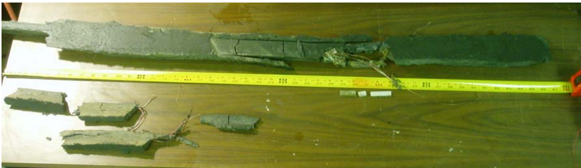
Figure 82 Recovered sensor assembly from Rt. 287 field installation.
