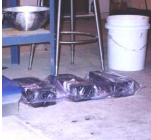
Figure 22 Photograph of the three bricks, with three separate epoxy samples each wrapped in saran wrap and sealed in plastic bags.
