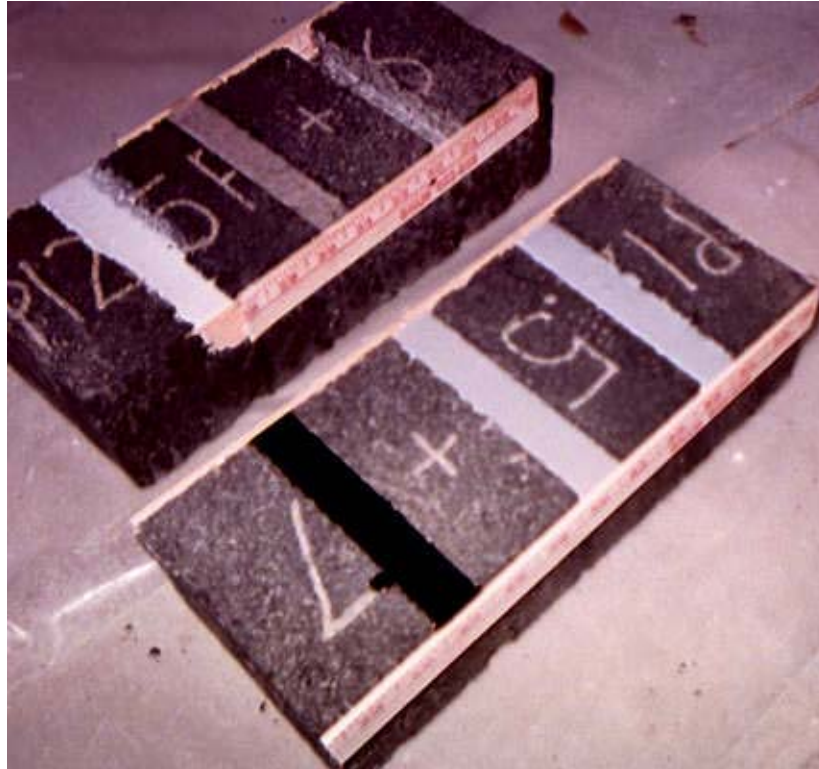
Figure 9 Photograph showing epoxy infiltration into the grooves previously cut into the HMA bricks.
