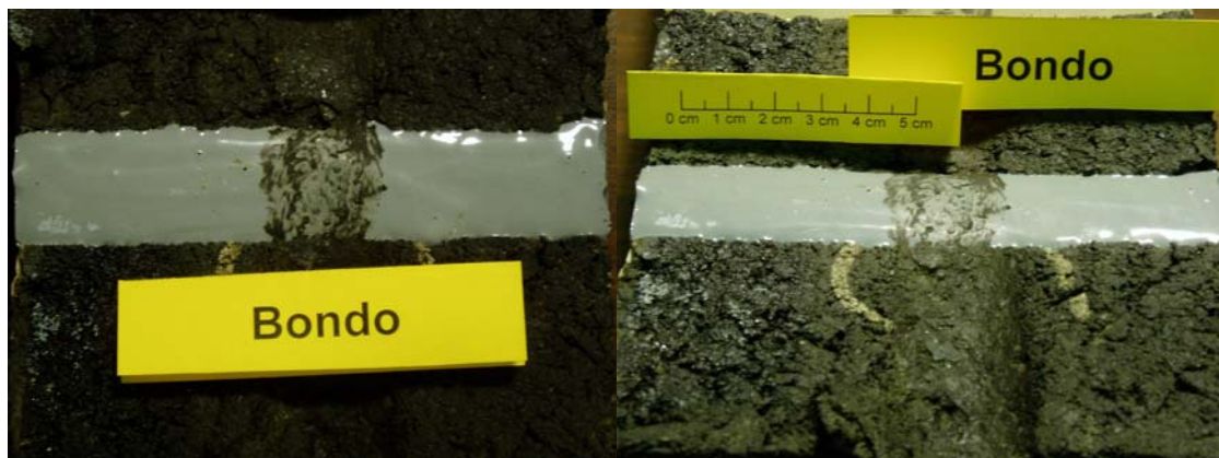
Figure 17 Photograph of APA Test rutting results of Bondo 7084.
