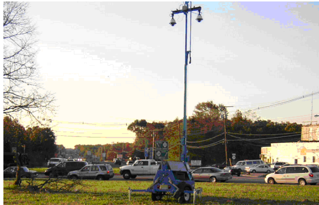
Figure 4. Portable tower video surveillance system (POGO)
