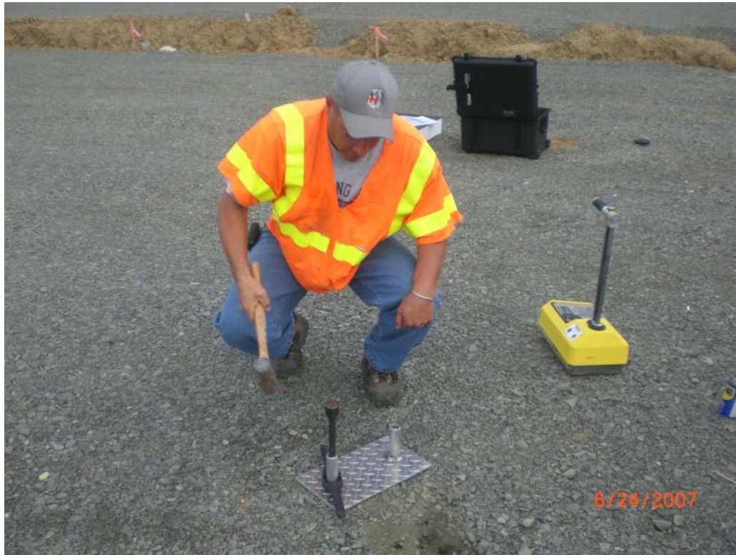
Figure 11 – Nuclear Gauge Setup
