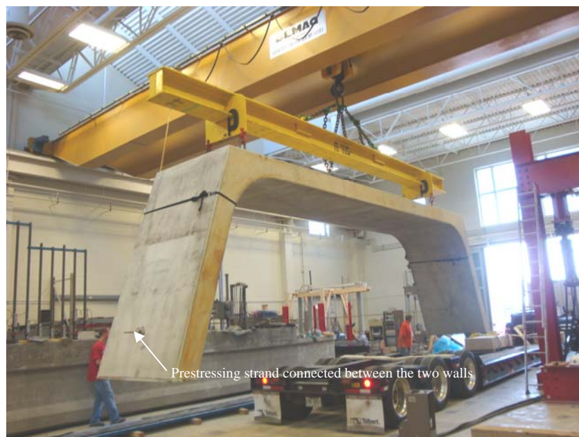
Figure 3.1. Handling of the Test Specimen in the Laboratory showing the Prestressing Strand Connected between the Two Inclined Legs
