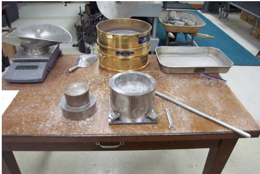
Figure 3: Missouri S&T ACV mold, rod, and plunger
