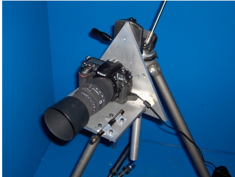
Figure 1: Sensor section of the HRTMM including the Nikon D200, Sigma lens, targeting laser, sensor platform, and video tripod head all mounted on a tripod.
