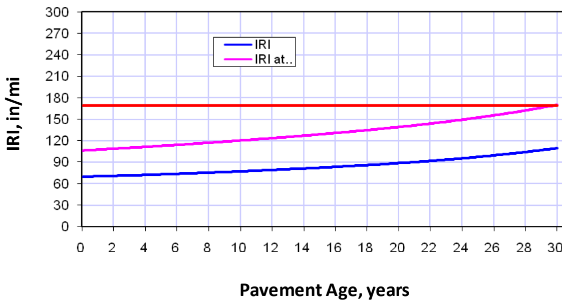
Figure B-19. Plot of predicted IRI versus pavement age.
