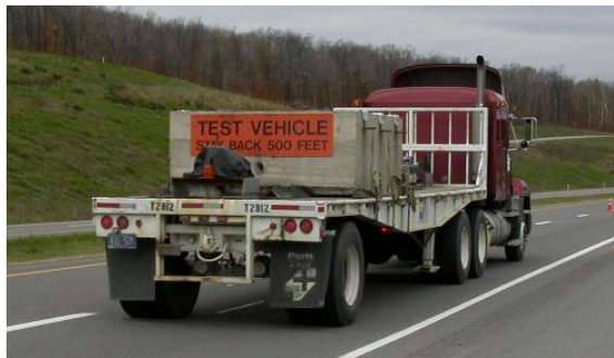
Figure 7. Truck with moveable weights for pavement loading.
