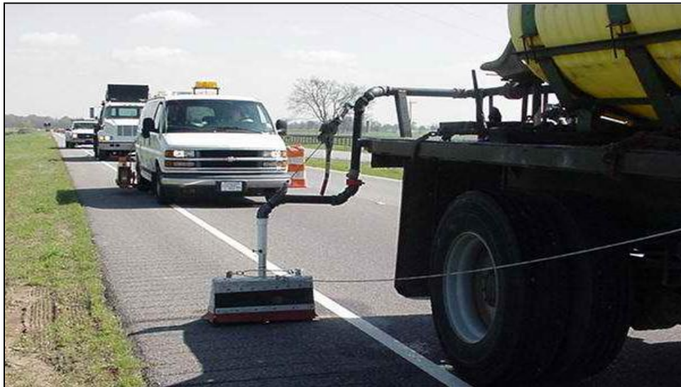
Figure 3-2. Wet test train of water truck, Laserlux, and attenuator truck.
