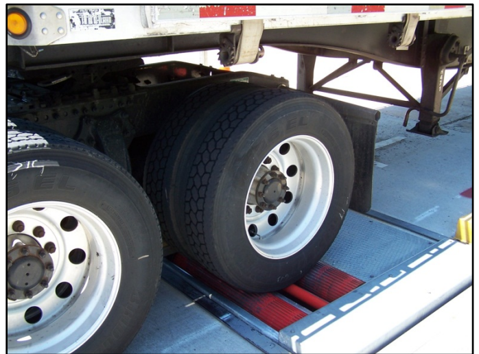
Figure 1. Image. PBBT located at the Greene County Inspection Station.
