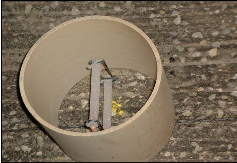
Figure 3.5: Strain Gages and Fixtures Setting
