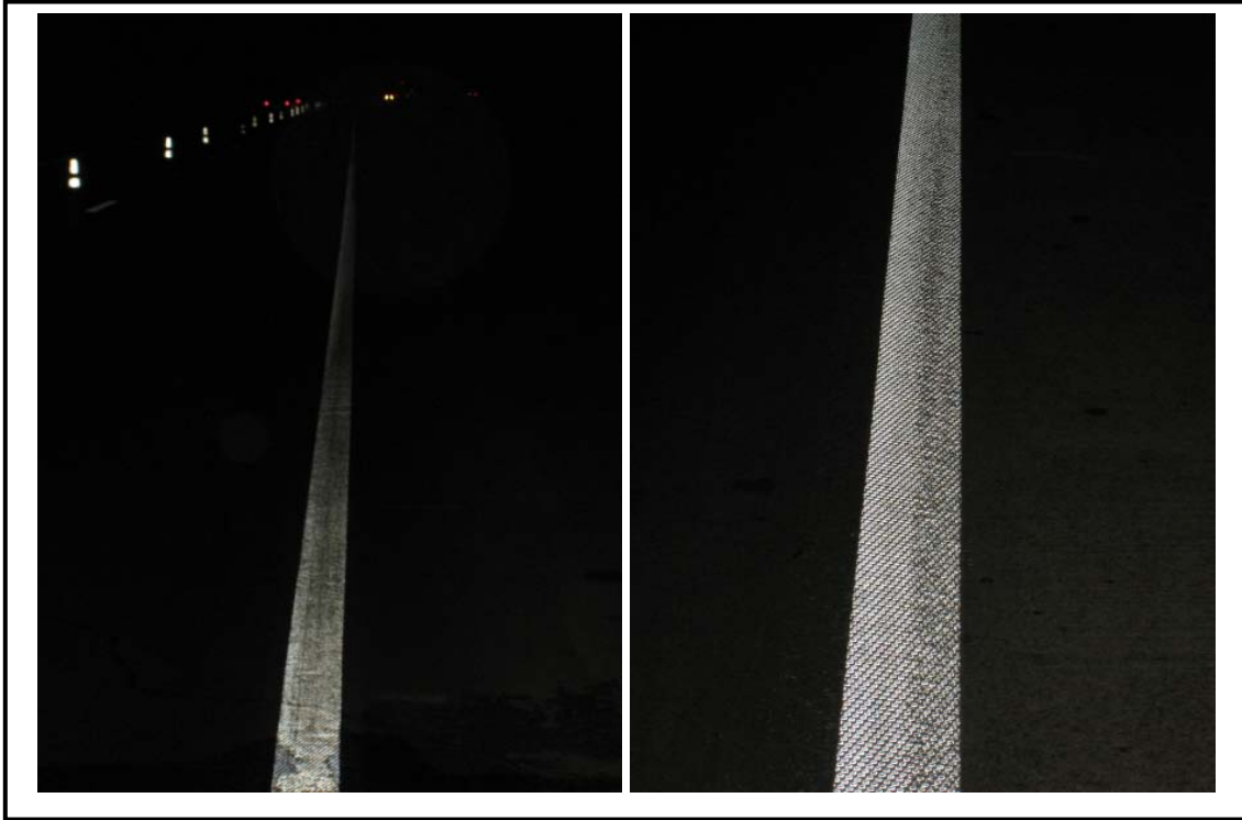
Figure 6. Uneven Wear on Section 5 Westbound Tape.
