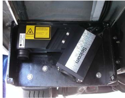
b) 64 kHz Laser Mounted on Truck.
