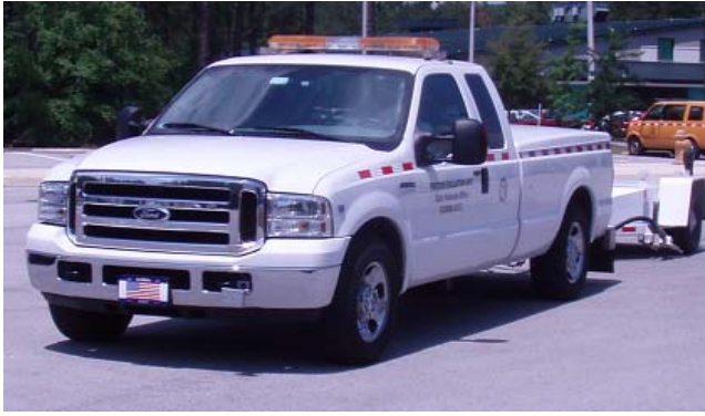
a) Florida DOT Locked-Wheel Friction Test Unit.
