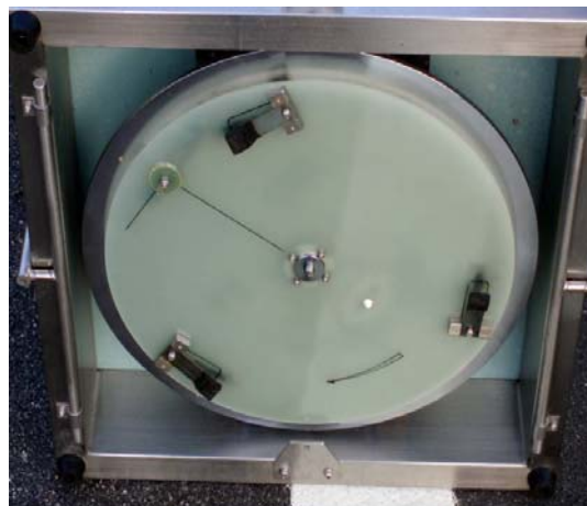
c) DFT Rubber Slider Pads.
