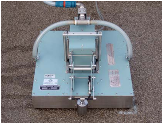
a) Dynamic Friction Tester (DFT).
