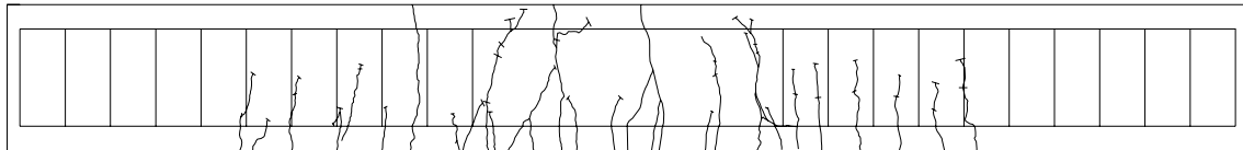
Figure 58: GE-F Eastern Face Crack Pattern
