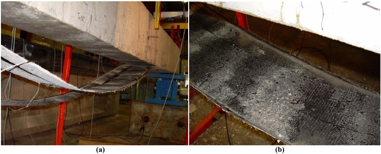
Figure 61: GE-F Specimen at Fail and Post-fail
