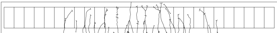
Figure 51: EP-F Eastern Face Crack Pattern
