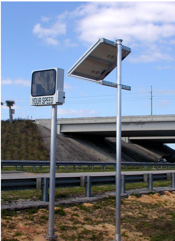
Dynamic speed monitoring system prototype
