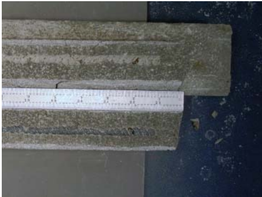
Figure F10: Photograph of the right bar and bar trace of Specimen 9B.
