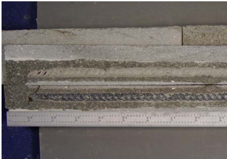
Figure F6: Photograph of the right bar and bar trace of Specimen 8B.
