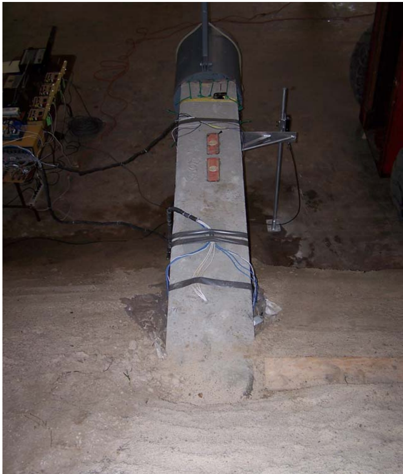
Figure 21. Pile imbedded in compacted soil and instrumentation set-up.
