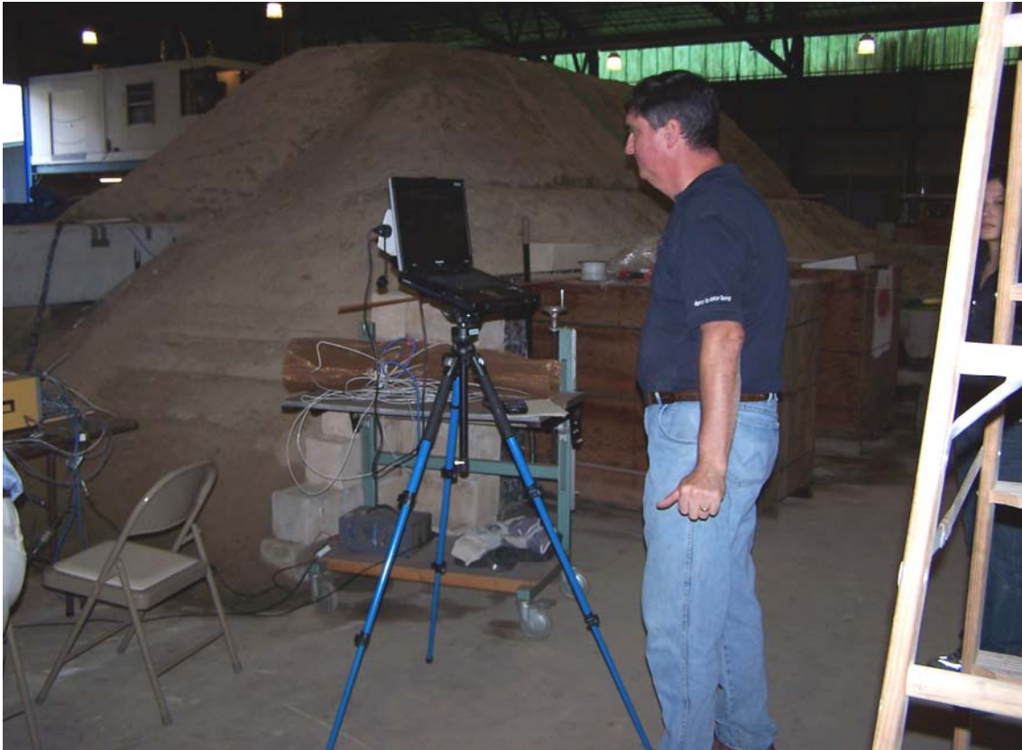
Figure 23. EDC pile wireless data collection set-up.
