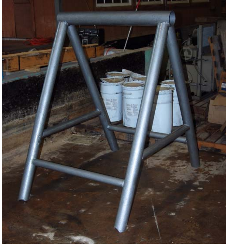
Figure 8. One of two stands constructed to support the horizontally suspended pile.
