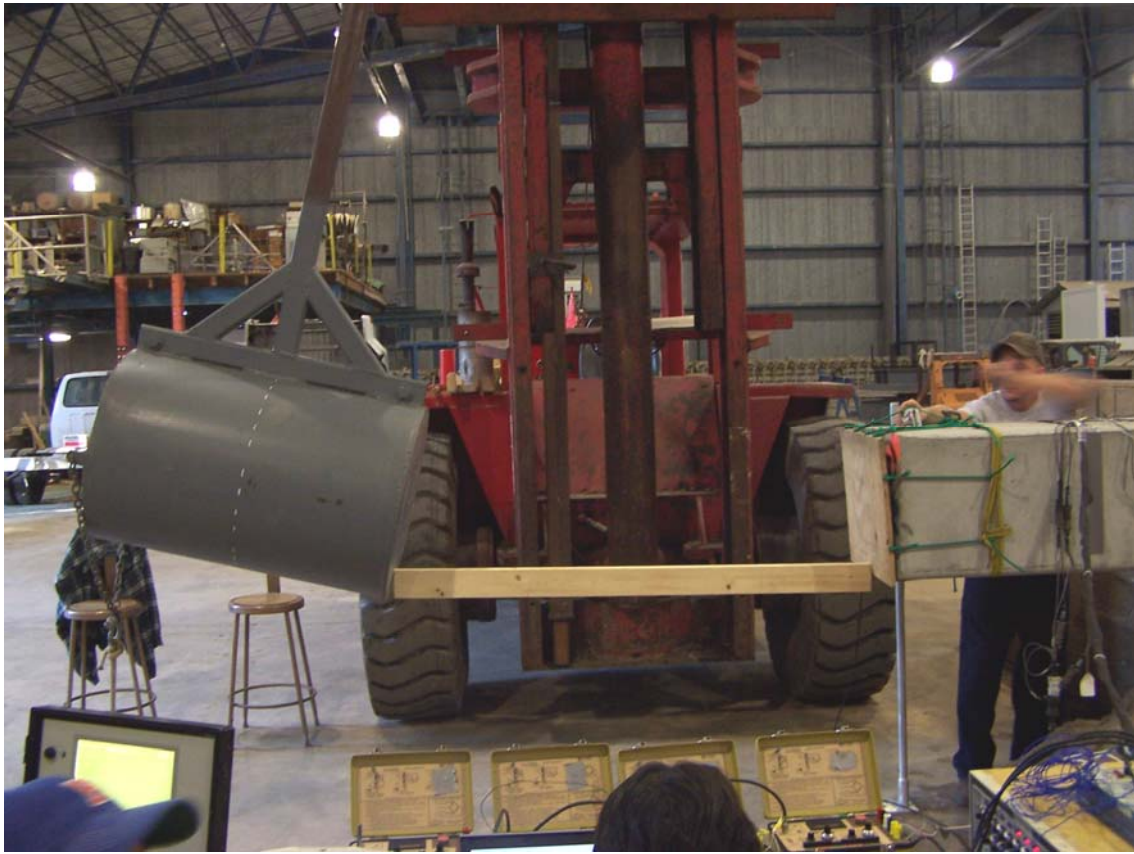
Figure 25. Pile impact hammer prior to release.
