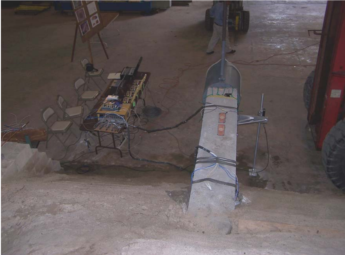
Figure 21. Pile imbedded in compacted soil and instrumentation set-up.
