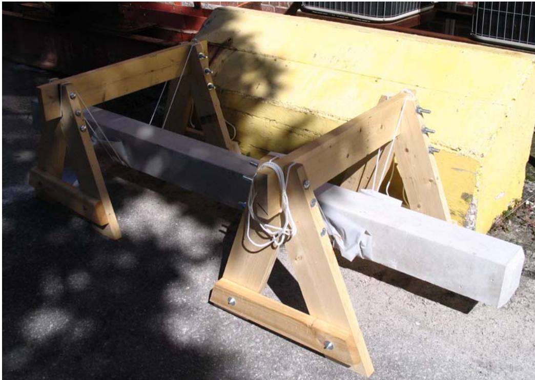
Figure 6. The PDA testing station of a horizontally suspended 6"×6"×8' concrete beam.
