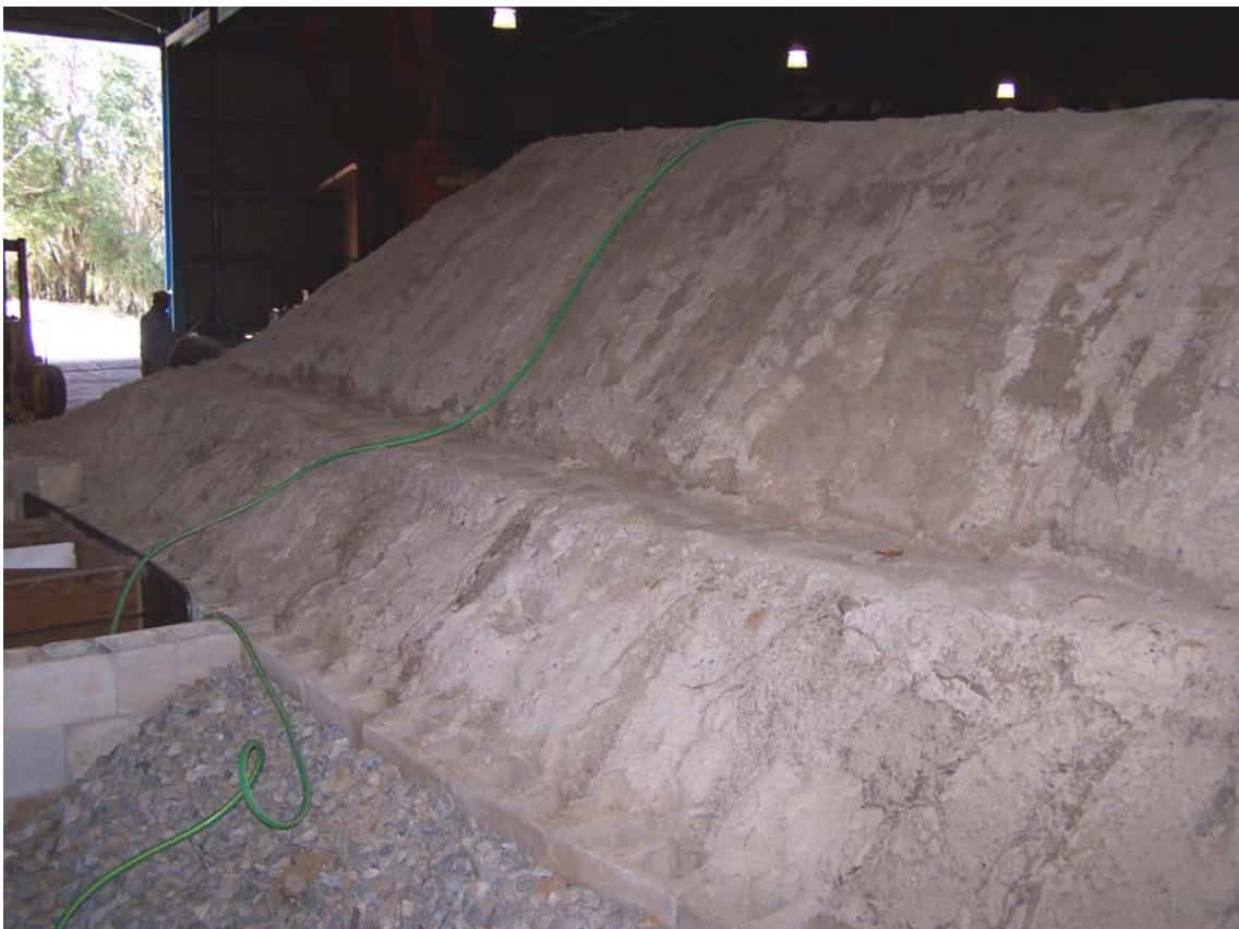
Figure 20. Zoned compacted soil.
