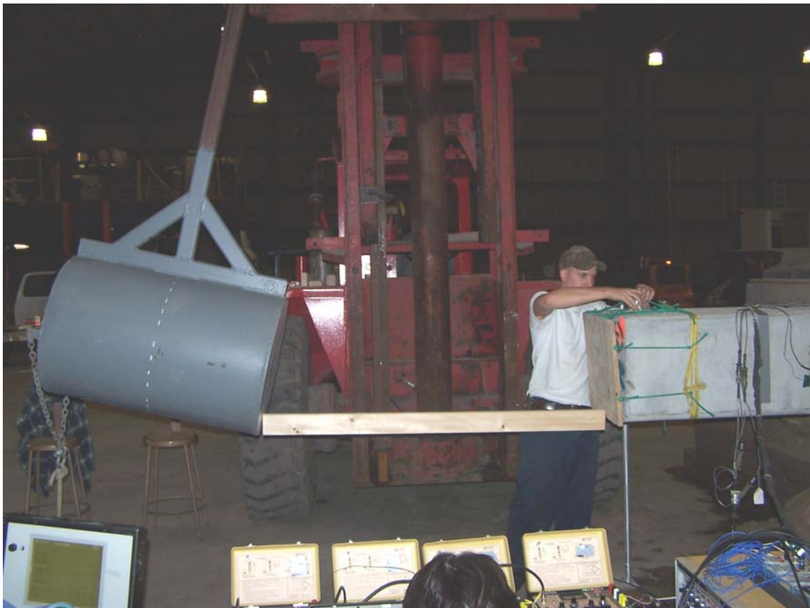
Figure 16. Impact hammer ready for release.
