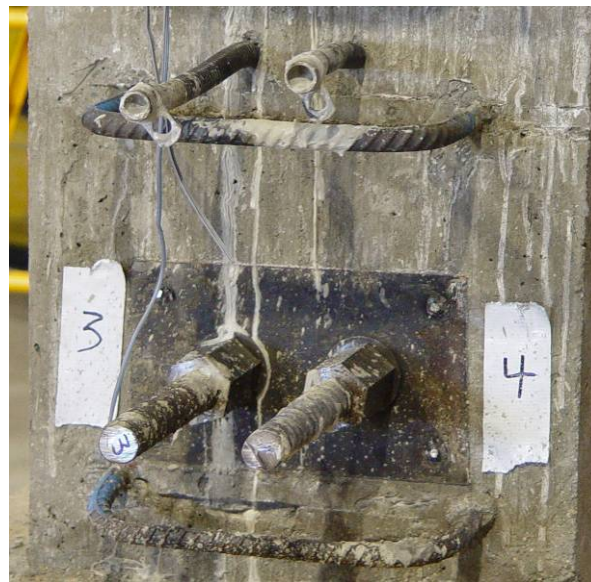
Figure 95 – Bottom anchorage including anchor plate, conical nuts, PT bar, and grouting tubes.
