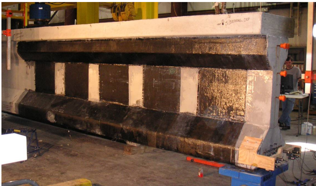
Figure 10 – Finished CFRP repair.
