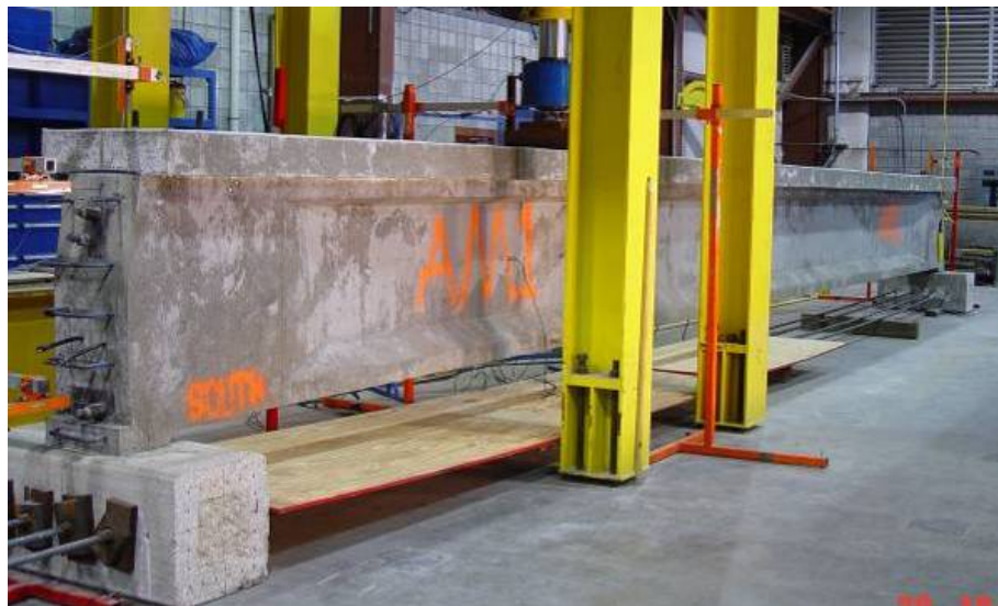
Figure 101 – Finished girder and deck.
