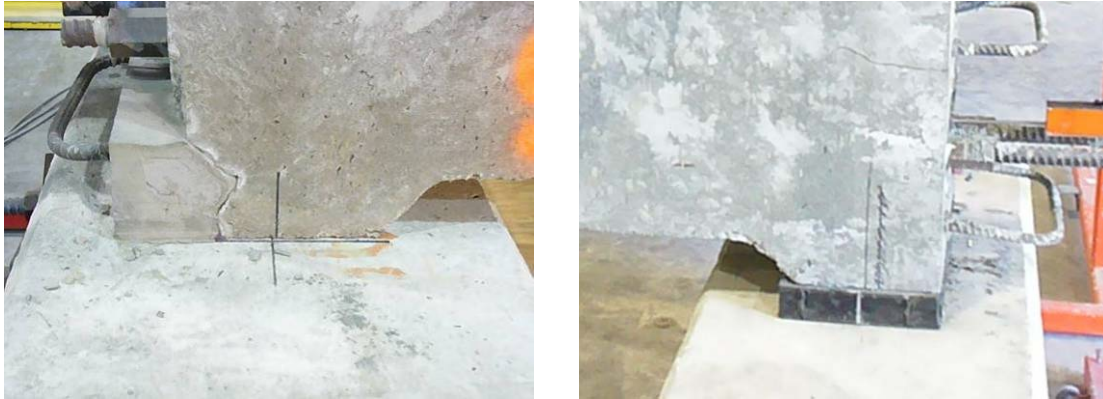
Figure 112 – Support Conditions, C1U3 (Left) and C2U3 (Right)
