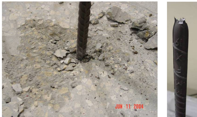
Figure 53. Bar condition after test (a) spalled concrete around base of bar and (b) rupture surface of bar.
