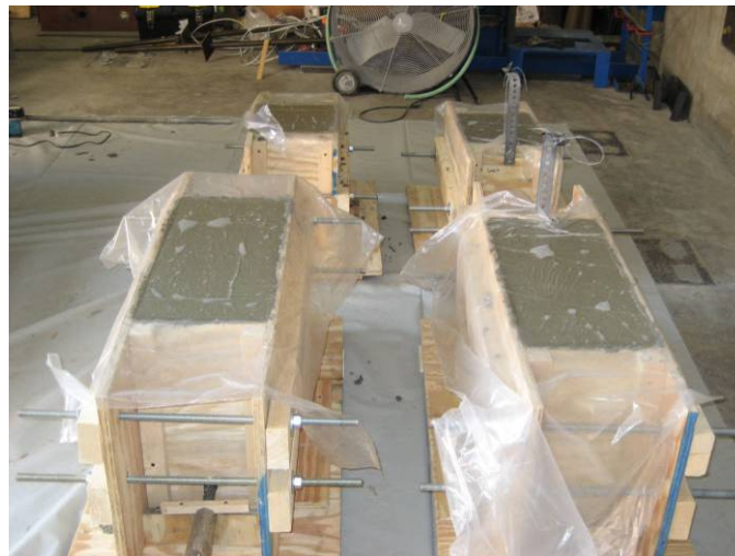
Figure 16. Curing of the specimens.
