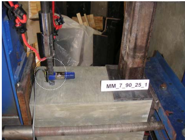
Figure 22. Linear potentiometer placement to measure bar strain.
