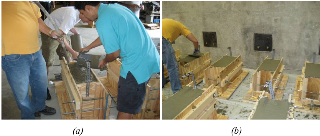
Figure 15. Casting and compaction of the specimen (a), and finishing of specimens (b).
