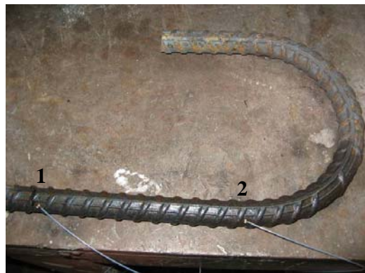
Figure 20. Positioning of slip wire in hooked bar.
