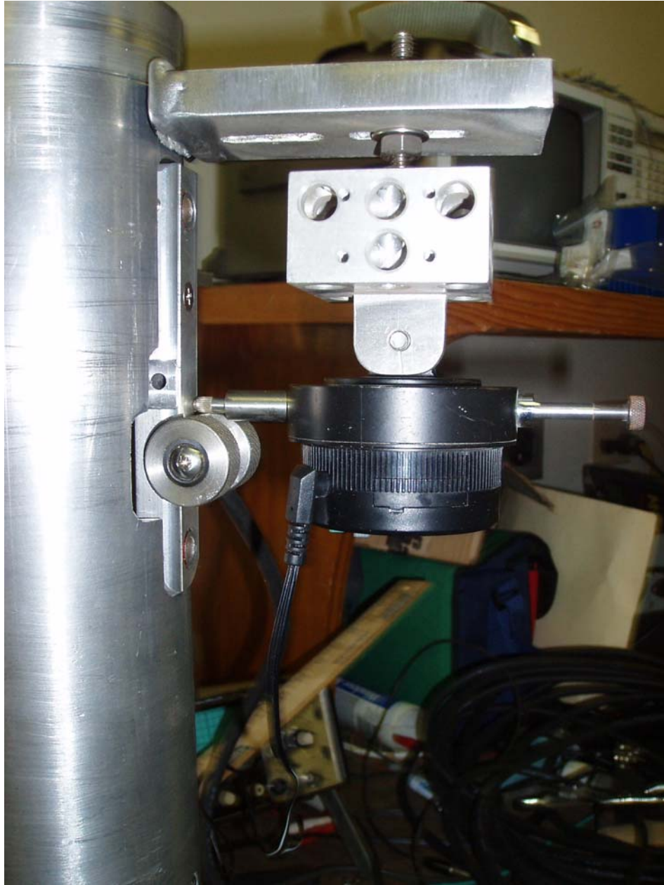
Figure 3-25. Air Cylinder Controlled Measuring Wheels During Calibration.
