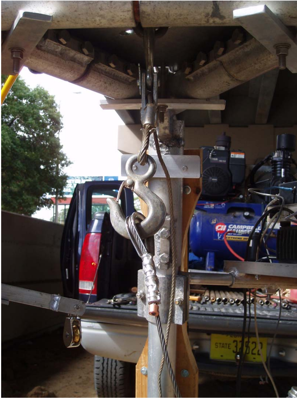
Figure D-13. Photo Showing Winch Cable and Pulley Setup on Tripod.
