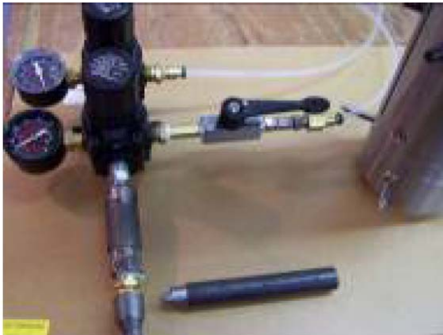
Figure 3-19. Compressed Air Supply Regulator.
