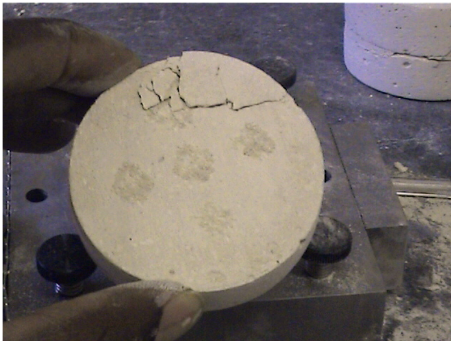
Figure 3-10. Sheared Multiple Head Gator Rock Sample Showing End Effects.
