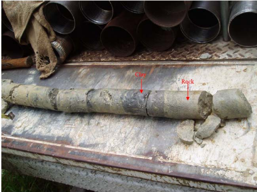
Figure 6-4. Core samples retrieved - note the clay intrusions.
