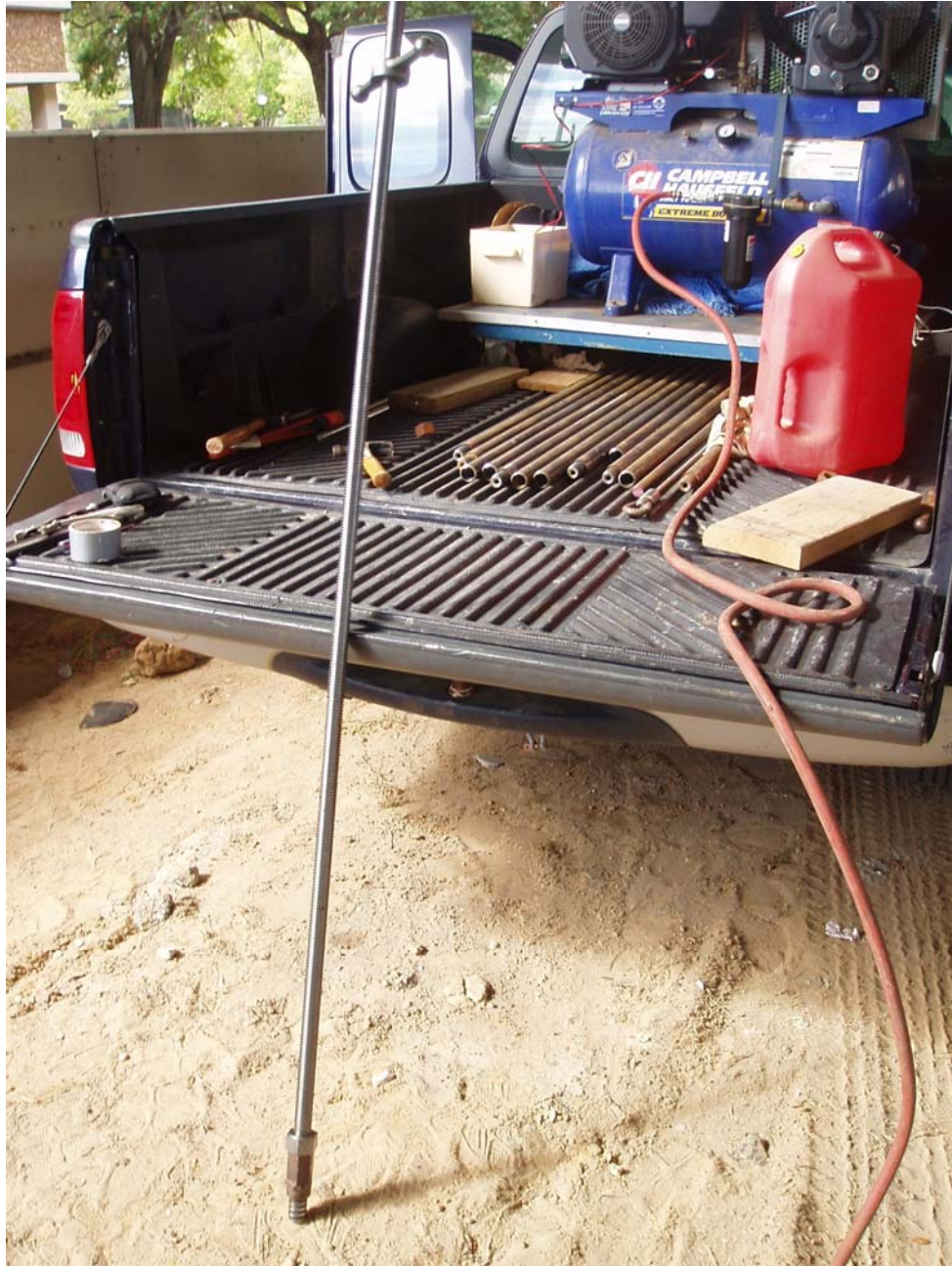
Figure D-6. 6 foot Threaded Rod used for Shallow Testing Depths
