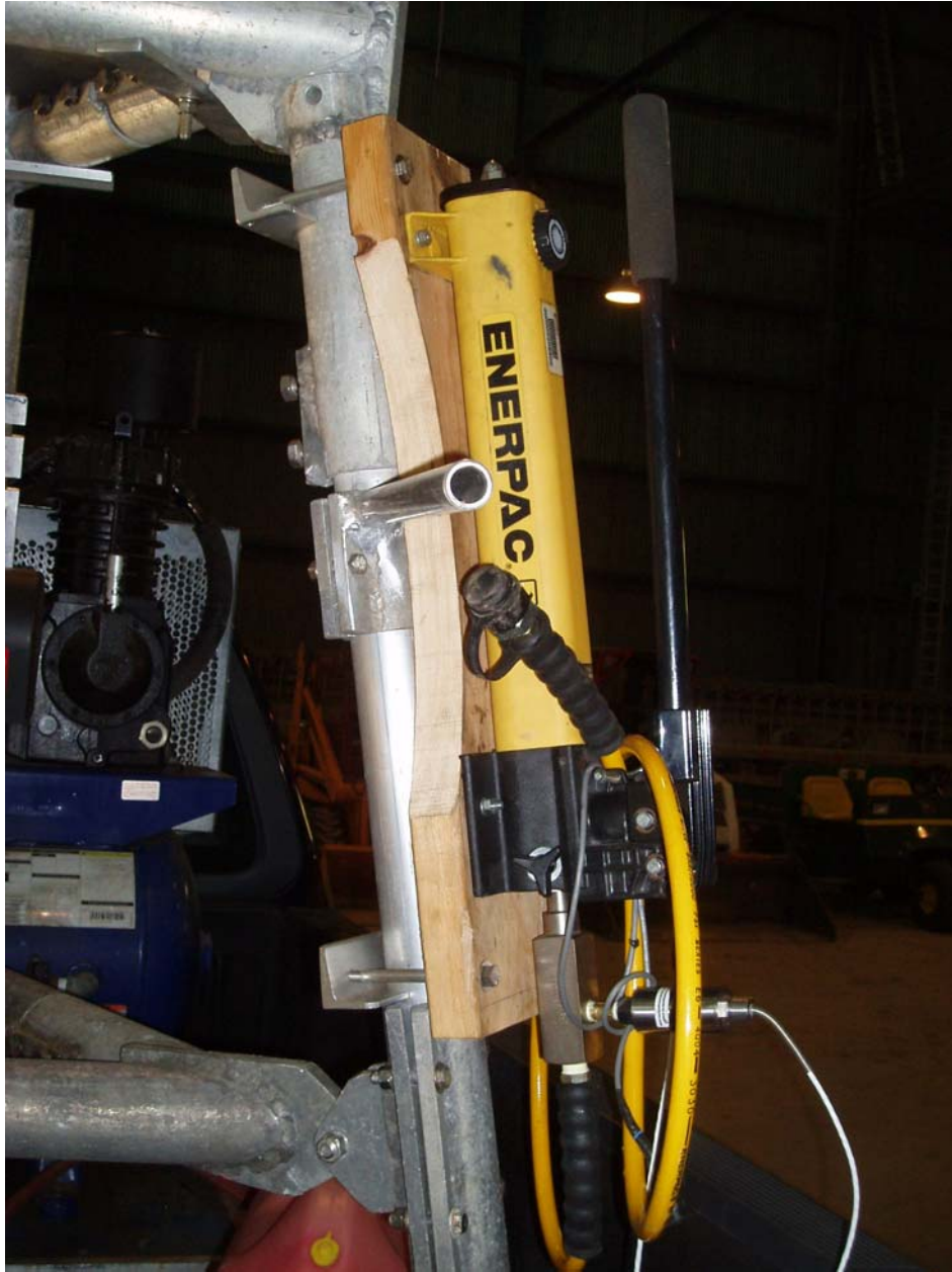
Figure D-3. Photo Showing Hydraulic Jack Connected to Leg of Tripod.
