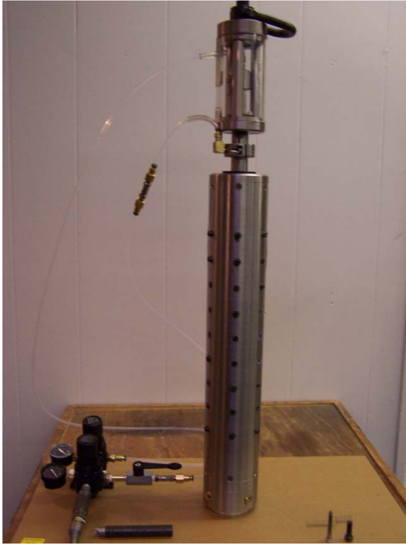
Figure 4-1. Rock Shear Device.
