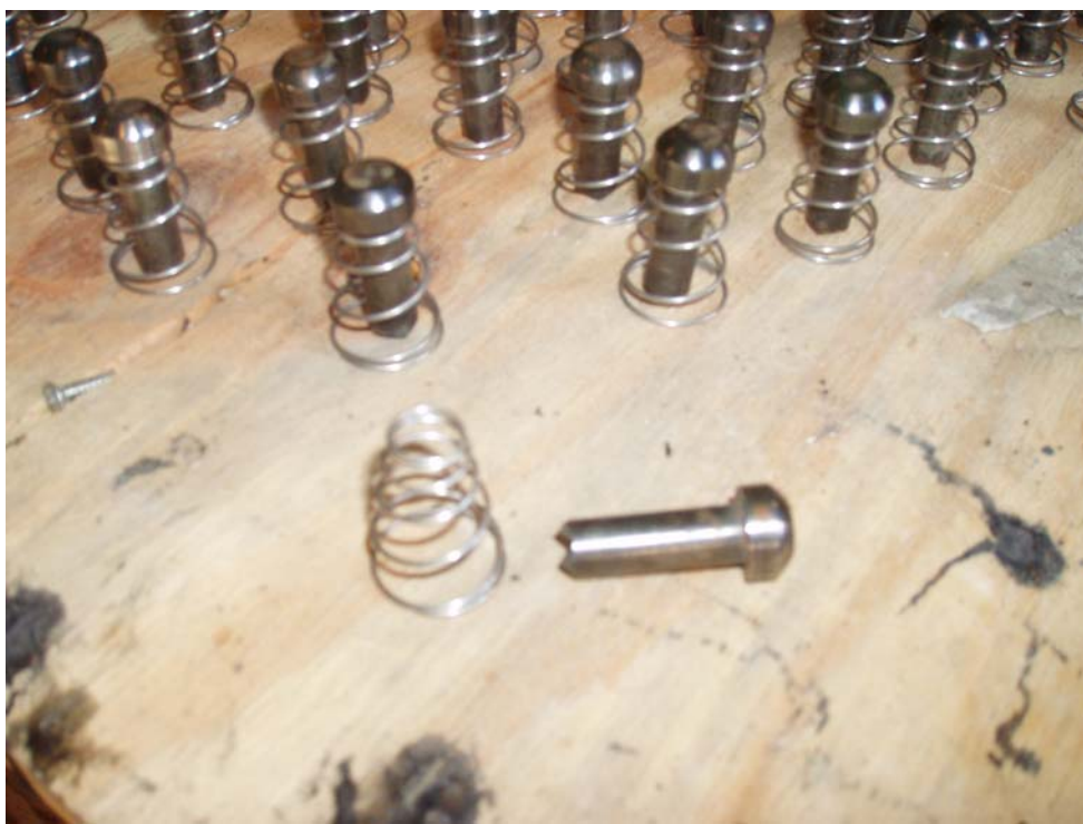
Figure D-15. Photo Showing Tapered Springs and on and off Studs.
