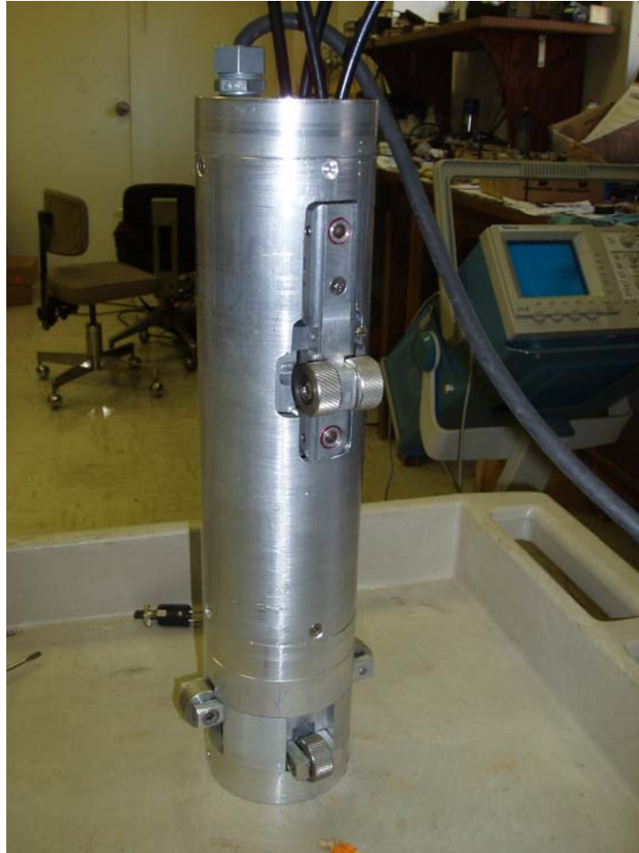
Figure 3-24. Corehole Mapping Device (CMD) Showing Measuring and Feeler Wheels.
