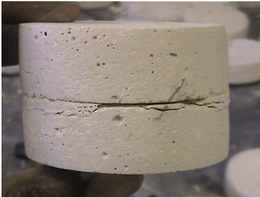
Figure 3-8. Direct Shear Sample Showing Predetermined Shear Plane.
