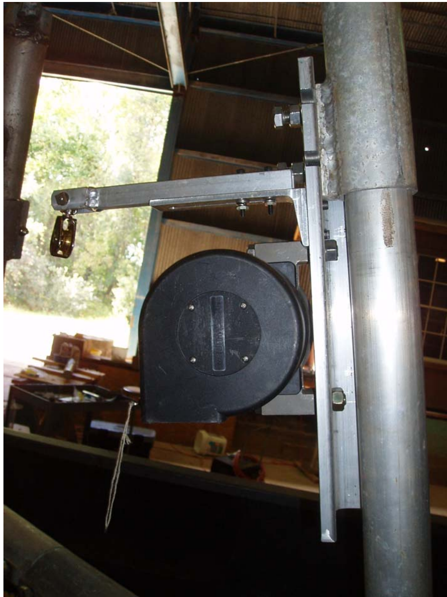
Figure D-20. Photo Showing String Pot and Pulley Connection.
