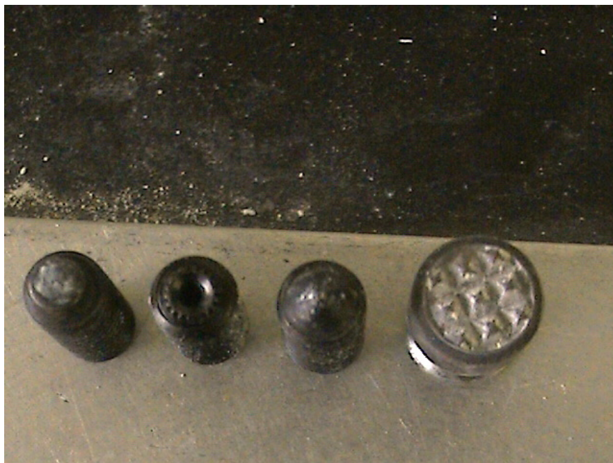
Figure 3-12. Shear Studs from left to right: Flat Head, Serrated Head, Pointed Head, and Multiple Head.
