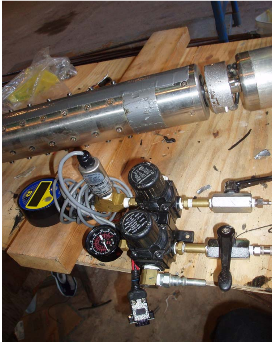
Figure D-9. Photo Showing Air Regulator with Pressure Transducer and Digital Dial Gauge and Electronic Connector to Black Box.
