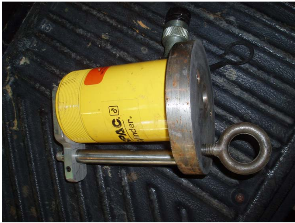
Figure D-19. Photo Showing Cylinder with Base plate, Closed Hook and LVDT.
