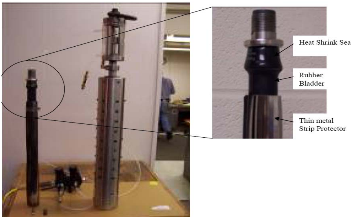
Figure 3-17. Probe and Inner Rubber Bladder/Chinese Lantern Assembly.
