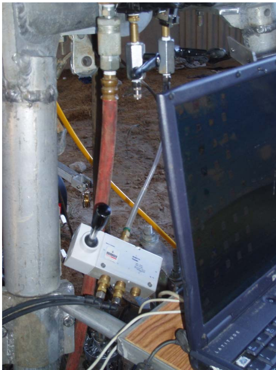
Figure D-22. Photo Showing Pressure Reversible Unit attached to Regulator.
