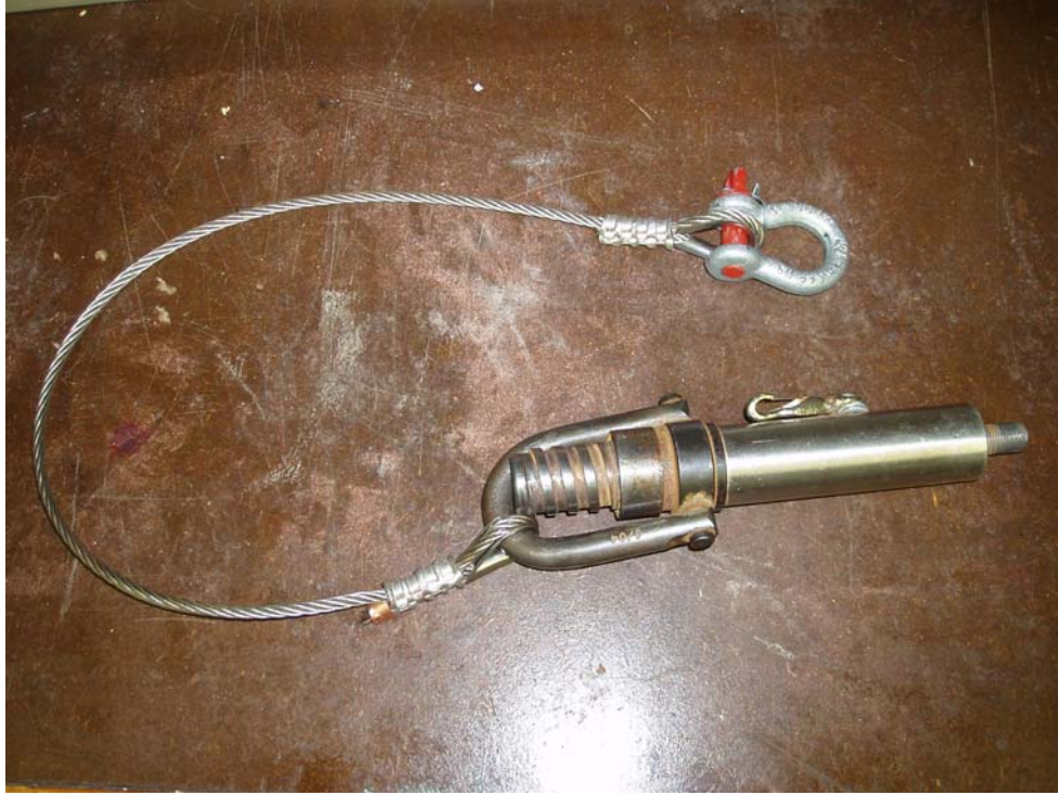
Figure D-7. Photo Showing Shear Device Adaptor with Cable and Connector.
