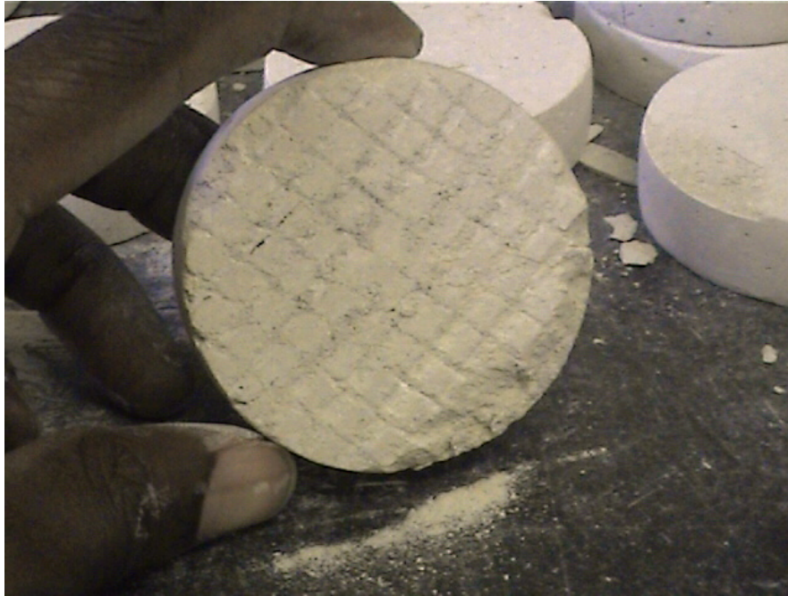
Figure 3-9. Sheared Wire Mesh Gator Rock Sample Showing some Edge Effects
