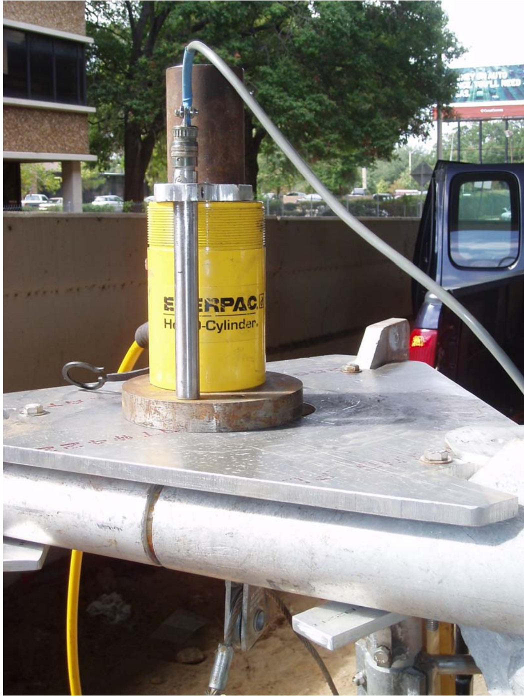
Figure D-21. Photo Showing Jack and LVDT with Steel Base Plate attached to Tripod Top.
