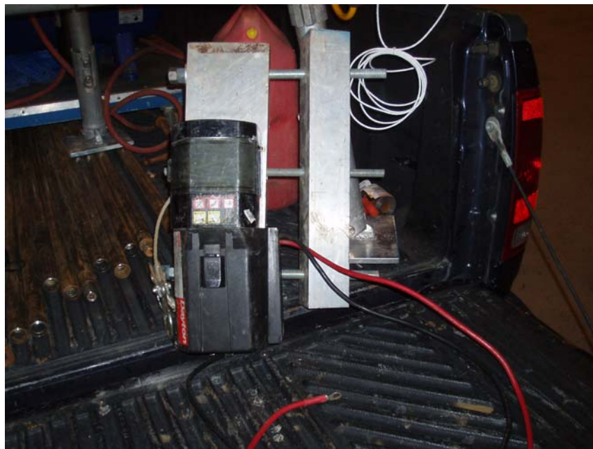
Figure D-4. Photos Showing Remote Controlled Winch with Tripod Connector.
