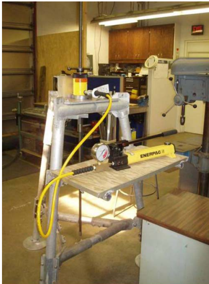
Figure 3-21. Tripod, Hydraulic Jack and Rod Setup.
