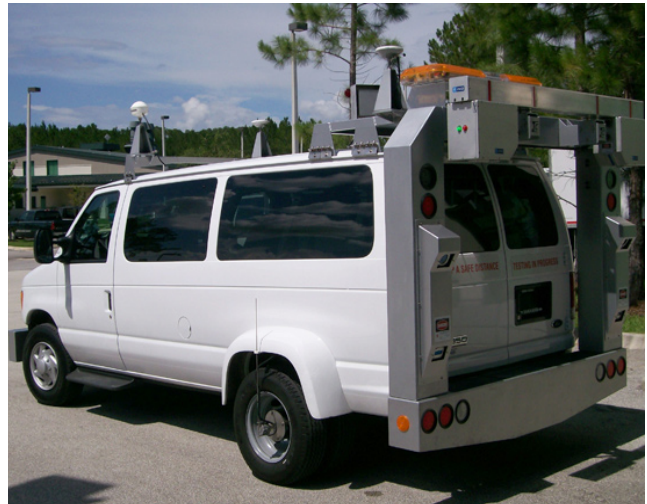
FDOT's Multi-Purpose Survey Vehicle uses image scans to evaluate highway conditions.
