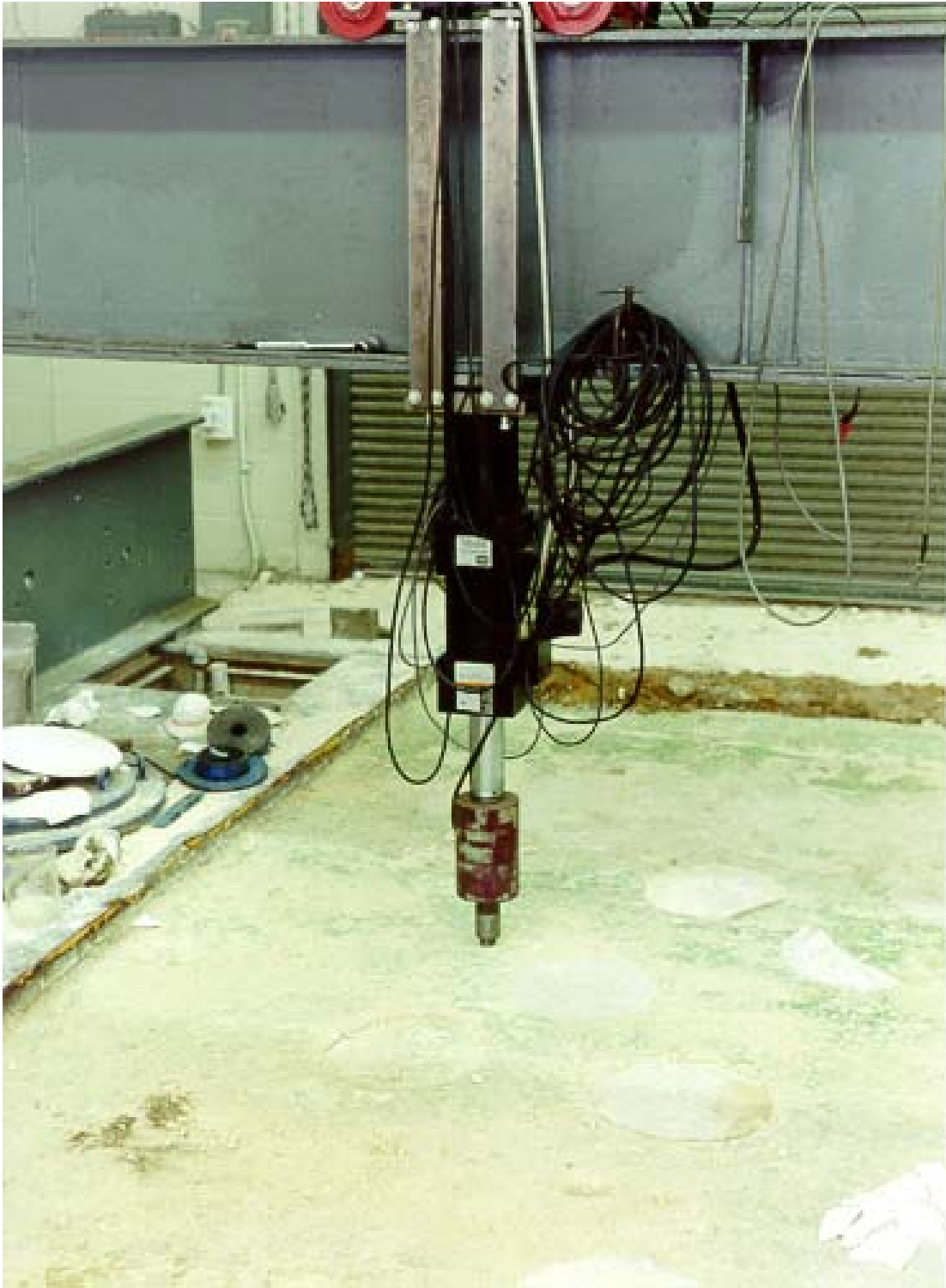
Figure 3.20 An Actual View of Test-Pit Loading System
