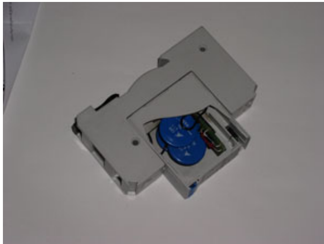
Figure 12. Damage to CITEL DS210-12VDC Suppressor
