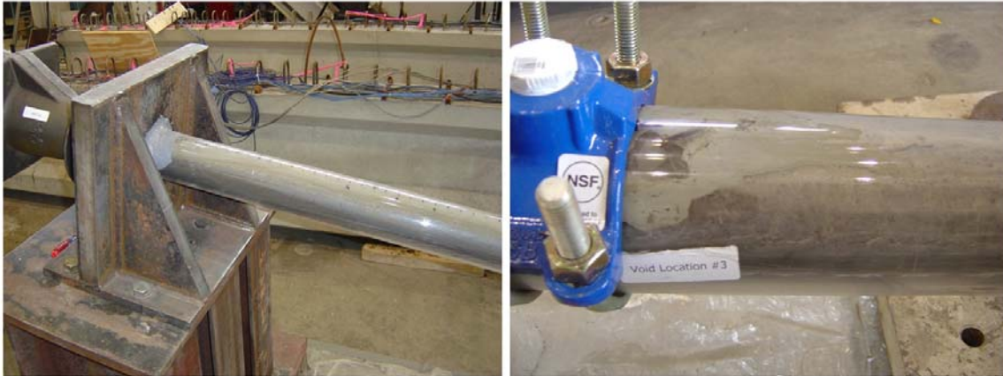
Figure B-5. Repair Grouted Ducts of Specimen VG-C2-1.
