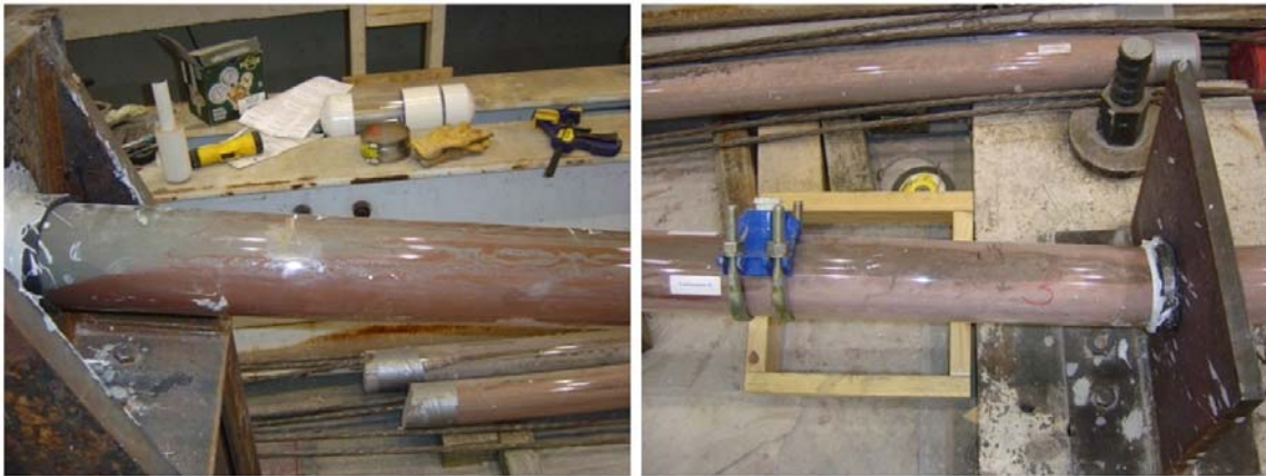
Figure B-31. Repair Grouted Ducts of Specimen PVG-C1-1.
