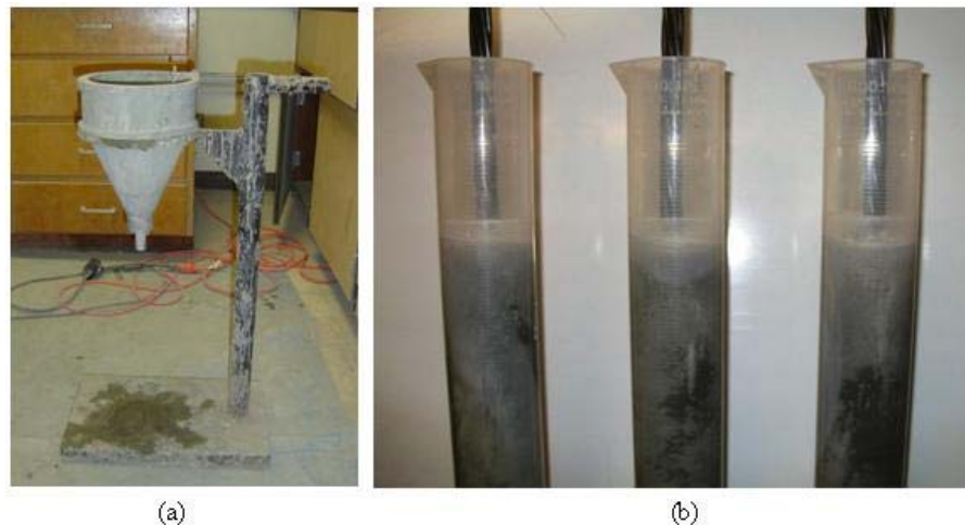
Figure 5-3. Flow Cone (a) and Wick-induced Bleed Test (b).
