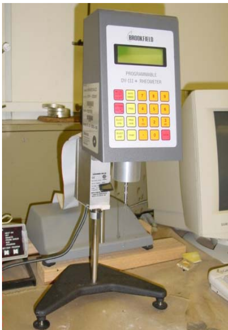
Figure 4-4. Brookfield Rheometer and Helipath™ Stand Used for the Viscosity Test.
