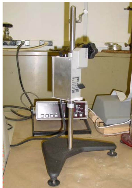
Figure 4-4. Brookfield Rheometer and Helipath™ Stand Used for the Viscosity Test.
