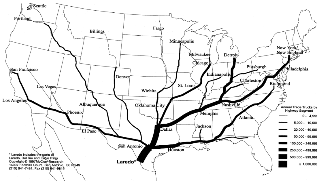
Figure 2-20. Estimated Trucks Carrying US-Mexico Trade on US Highway Corridors to and from the Laredo Region (McGray 1998).
