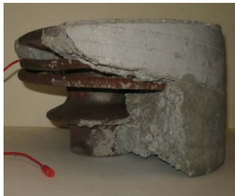
Partially-cast specimen showing the bearing plate and spiral reinforcement
