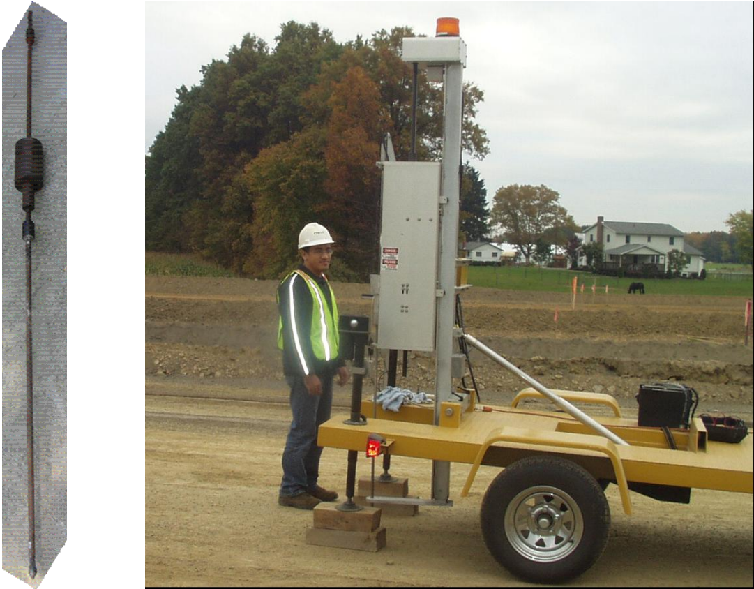
Color Plate 2. DCP test device: at left is the DCP rod and driving weight assembly, and on the right is the DCP in use. [Wu and Sargand, 2007]. See Figure 5.
