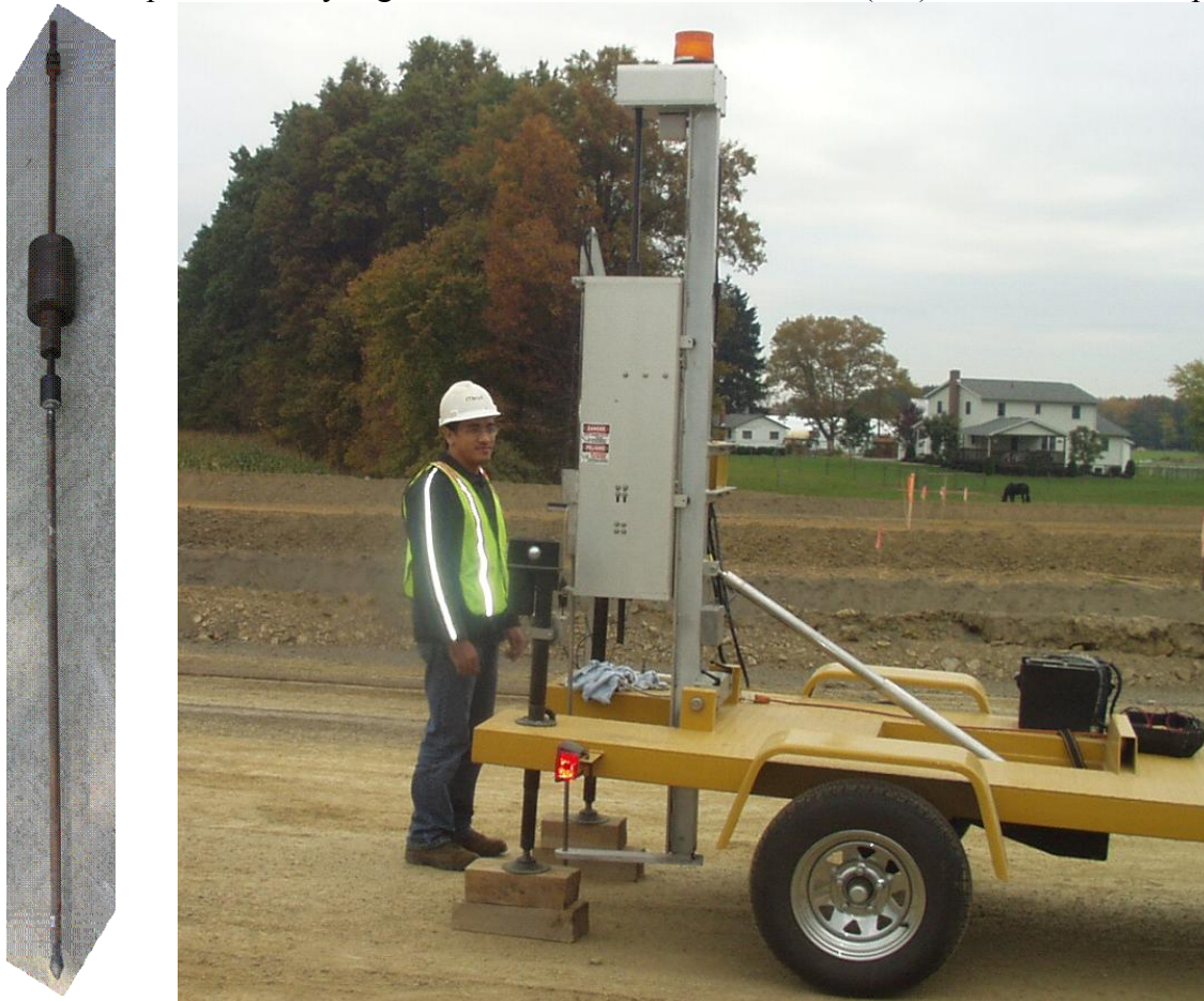
Figure 5. DCP test device: at left is the DCP rod and driving weight assembly, and on the right is the DCP in use. [Wu and Sargand, 2007]. See Color Plate 2 in Appendix E.
