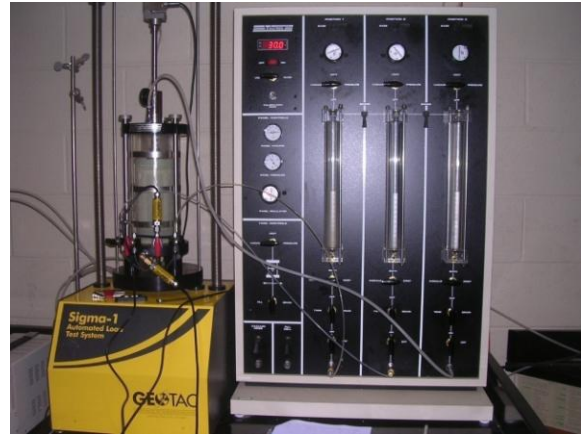
Figure 3: C-U Triaxial Compression Test Running at ORITE Laboratory
