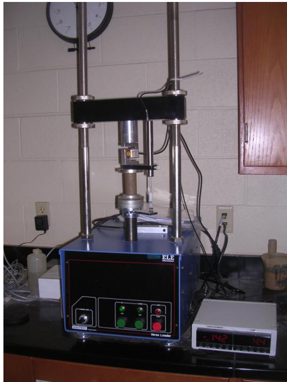
Figure 3.3: Unconfined Compression Test Machine
