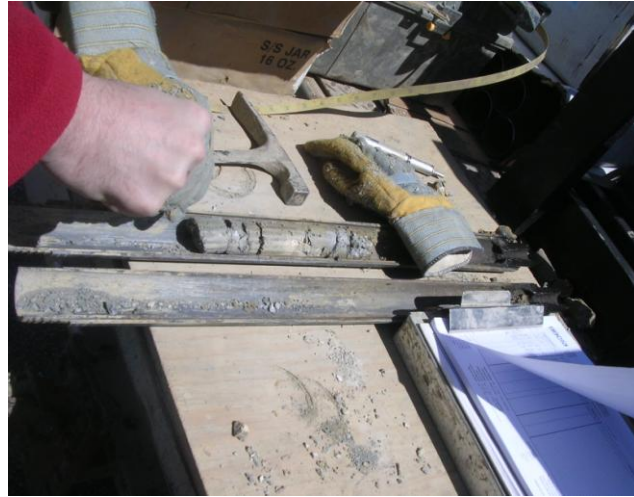
Figure 2.7: Split-Spoon Sampler (detached from the drill rig with soil sample inside)
