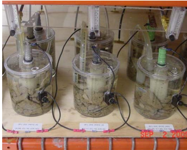
Figure 5. Rapid Macrocell Test Setup on the Rack.
