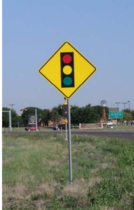
Figure 6. Signal Ahead Sign (W3-3) without Beacons.
