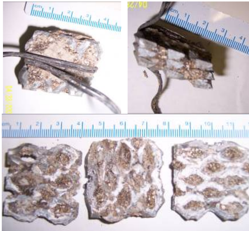
Figure 2b - Type W anode specimens. Zinc alloy anode appearance after embedded mortar was stripped. Top group of pictures, 1st set. Bottom group, 2nd set (mortar only partially stripped).
